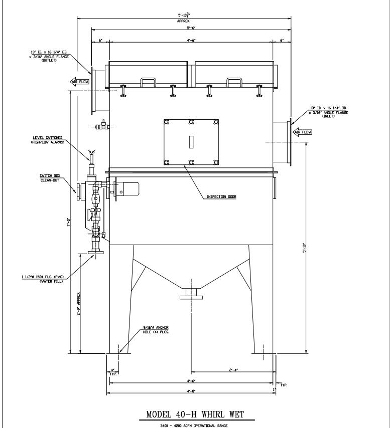
3400 - 4200 ACFM OPERATIONAL RANGE 10 GA. MILD STEEL WELDED CONSTRUCTION EPOXY PAINT 'TRI-MER' BLUE
