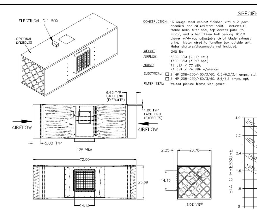
PREFILTERS; (2) 4" Pleated std. MAIN FILTERS:  $\square$  (2) 66 ft  $^2$  multi-pocket 65%, std. ☐ (2) 95% - opt, (2) Easy clean, opt. (2) 83 ft, 2 multi-pocket 65% (3 HP option)  $\underline{\text{OTHER OPTIONS:}} \ \square \ \text{Pressure gauge kit indicates filter changes}$ ☐ Mounting eye-bolts.
