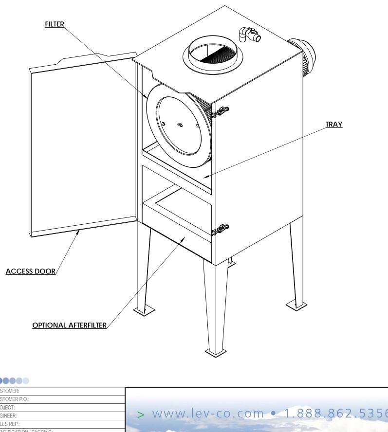
MAIN FILTER BOX DIMENSIONS: WIDTH: 18-1/16" DEPTH: 14-7/16" HEIGHT: 16-3/4" **OPTIONAL AFTERFILTER BOX DIMENSIONS:** WIDTH: 18-1/16" DEPTH: 20-1/4" HEIGHT: 12-3/4"
