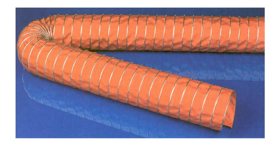
Special-coated high temperature fabric, asbestos free, reinforced by woven in stainless steel wire; external helix of galvanized steel
